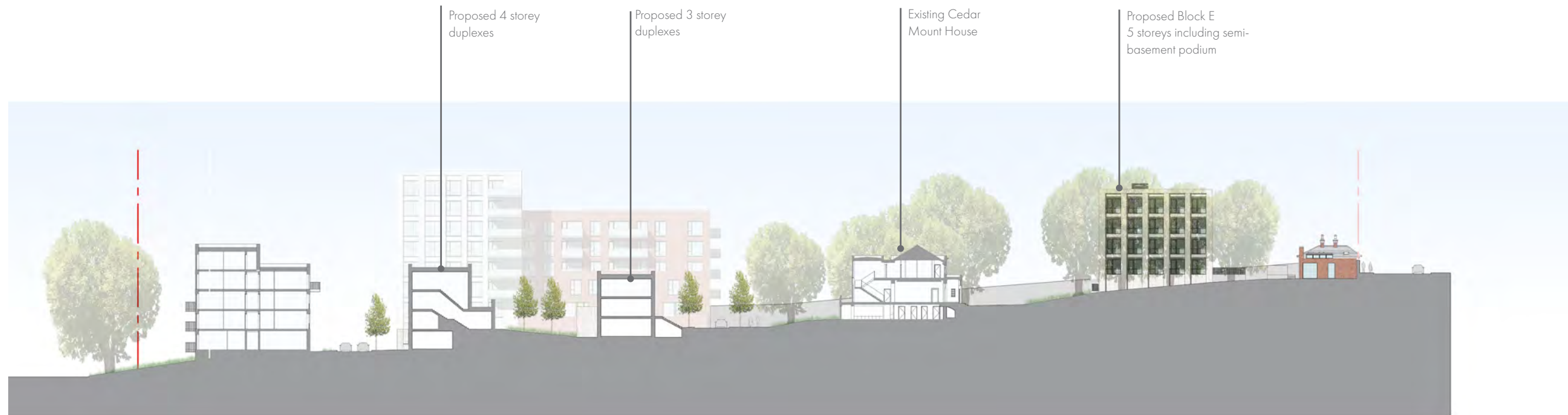
Section CC, showing Cedarmount House (3 storeys), Block E (5 storeys including semi-basement podium) and duplexes (3 storeys and 4 storeys); Existing trees that are between 15-17 metres provide screening between Cedarmount House and Block E.
